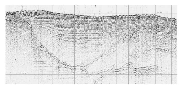
Figures 2 & 3: Shallow seismic section through an infilled palaeo-channel in about 30m of water, off the coast of Sussex
